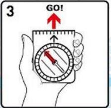
Hold the compass in hand and turn your body until the red end of the compass needle (North) coincides with the red arrow in the bottom of the compass housing. The front of the compass with the direction of travel arrow is now pointing towards your destination.
