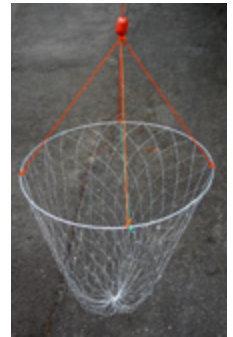
An example of a hoop or lift net – the ring and net lay on the bottom when set and crabs feeding on the bait are caught when the net is lifted.
